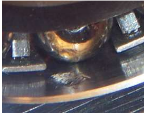
Fig. 1. Outer race defect of the rolling element bearing type EKTN9 [4]
